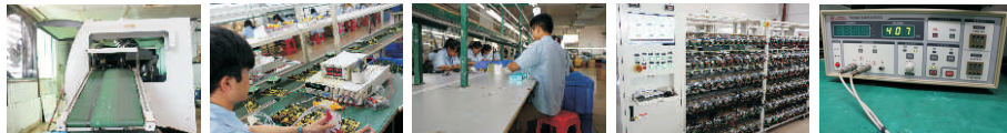
波峰焊 Wave soldering QC检测 QC Inspection 装配产线 Assembly production line 老化测试 Aging test 漏电流测试仪 Leakage tester
